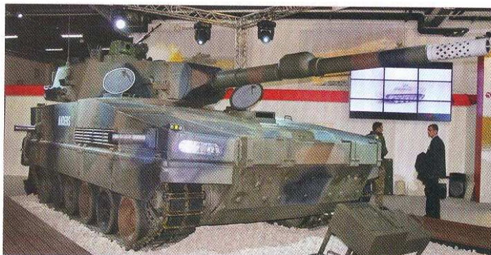
■ The Anders WWO fire-support vehicle demonstrator, showing the turret with its RUAG CTG 120 smoothbore gun and ZSMU Kobuz remote weapon station.
